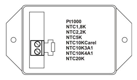
current output 4...20mA; power supply from the current loop
